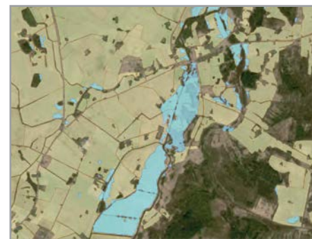
Flooded area mapped (blue) using Sentinel-1&2. Overlap with reference parcels (yellow) show the lost yield in Eastern Latvia. Credit: Contains modified Copernicus Sentinel data 2017
