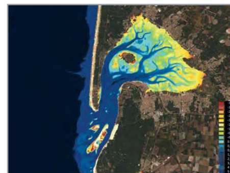
Satellite derived Bathymetry of the Arcachon Lagoon, derived from Sentinel-2A imagery. Optically deep waters are represented in black.
